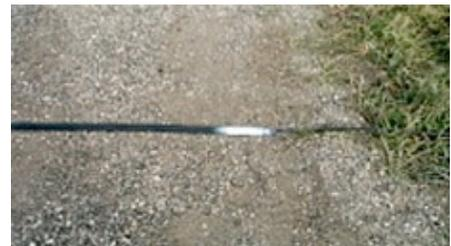
Stretch sensor taut across road. Secure sensor with second spike through second wire loop. Connect output end of sensor to traffic counter.
